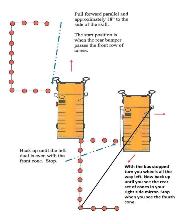
With the bus stopped, straighten your wheels and back straight until your reference point is just before the boundary line. Stop.
