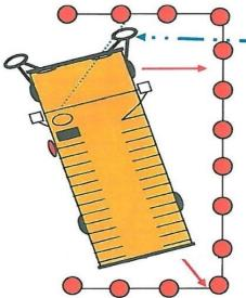
Watch the right crossover mirror as you back up in order not to encroach on the front row of cones. Continue backing up with the steering wheel turned left until the bus is parallel with the box line and stop.
