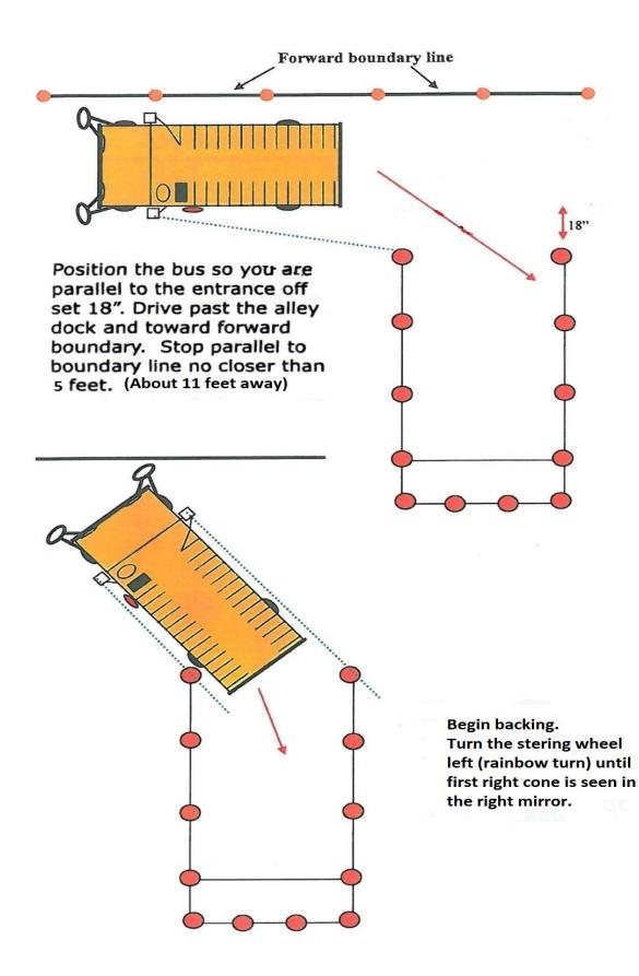
Straighten you wheels and backup. Turn slightly left or right as needed to position the bus between the cones.
