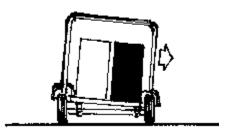
Heavy items loaded to one side of the trailer can cause oscillation or handling problems in turns.
