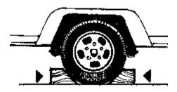
Whenever the trailer is detached from the tow vehicle, block the wheels so it is impossible for the trailer to roll off on its own. Better yet, do not ever detach the trailer on any grade.
