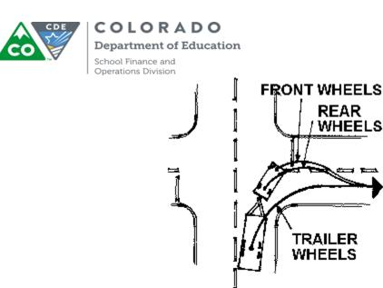
The longer the trailer, the wider you must swing in a turn to make sure the trailer wheels clear the inside curb.
