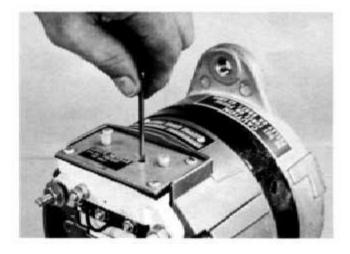
4. Turn the screwdriver clockwise to raise the voltage, counterclockwise to lower the voltage. Set the voltage between 14.0 and 14.2 volts (28.0 to 28.4 volts for 24-volt
